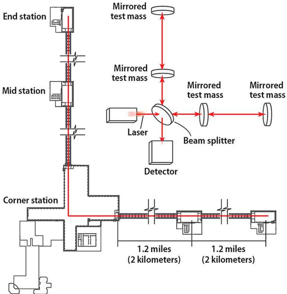
This diagram shows the layout of the observatory in Hanford, Washington. By making laser light travel up and down the arms and interfere with itself, scientists can deduce minute changes in the light's path from a gravitational wave encounter. *Astronomy*: Roen Kelly
